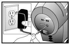
During long-term storage, the battery should remain permanently connected to the charger and the charger plugged into a power source. A microprocessor, inside the machine, monitors the battery and maintains a full charge.
